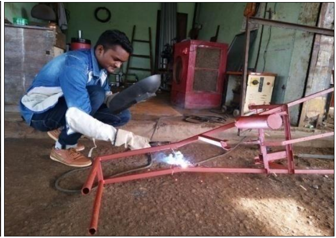
Fig 2: Welding to extended portion
