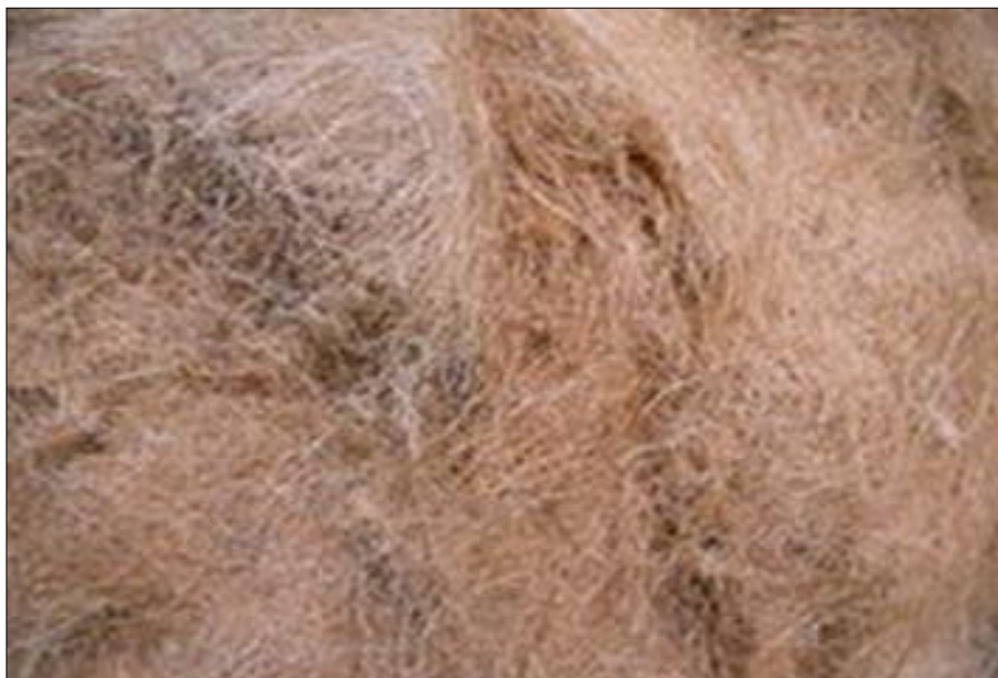
Fig 7: A close-up view of coir fibre
